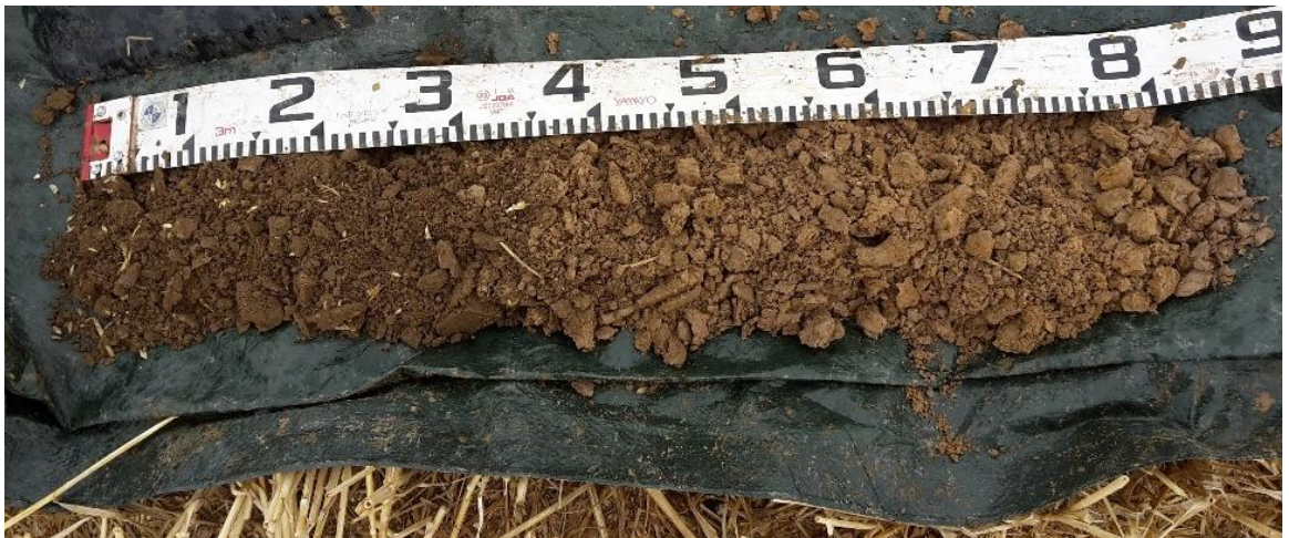
Photograph 20.1: Soil profile at the proposed converter station site sample point 11 (scale in decimetres), consistent with the Wisbech soil series of the Wallasea 2 soil association.
