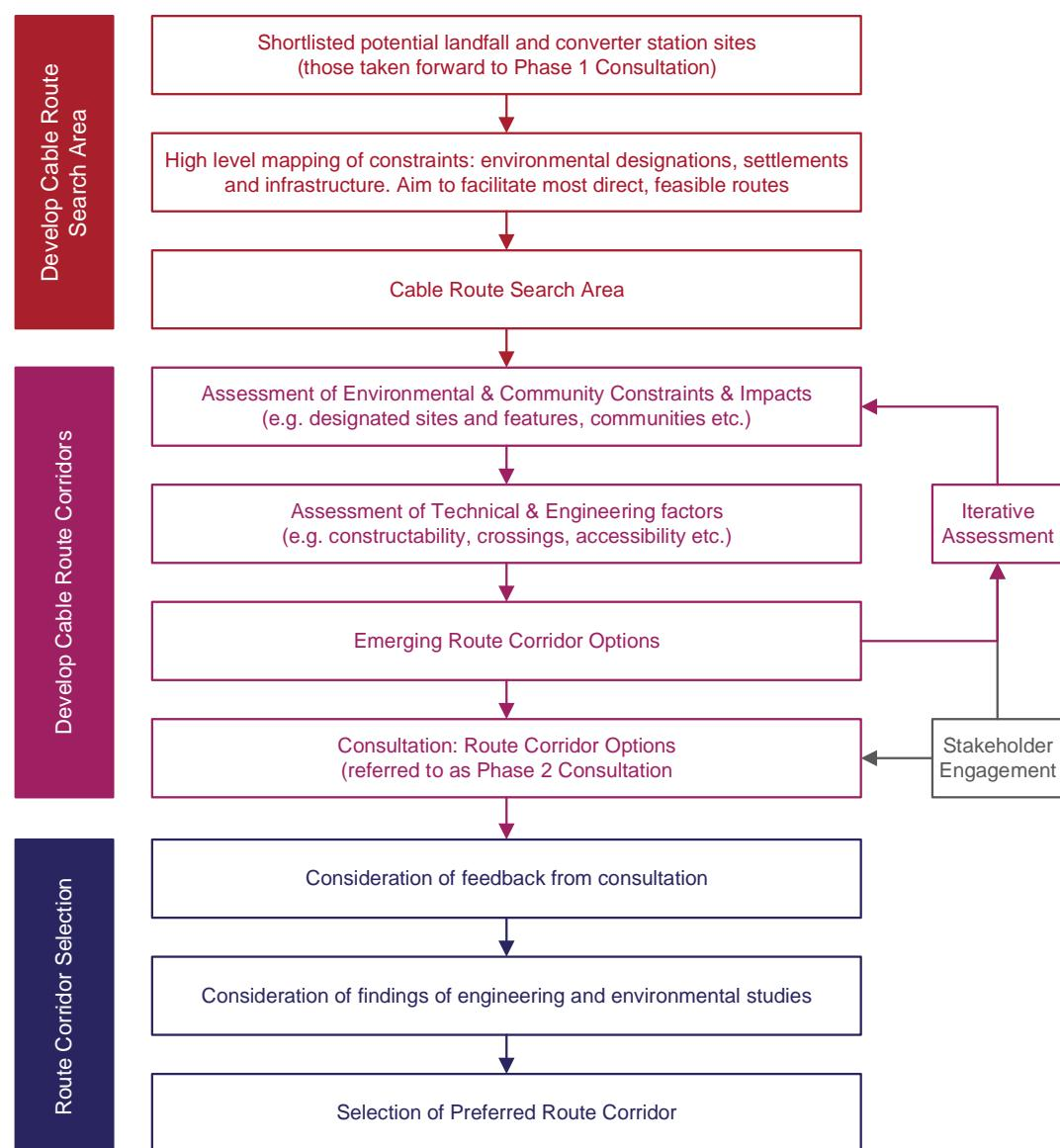
**Figure 2.10 Approach to Cable Routing**
